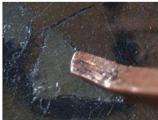
Fig. 7. Flattening of the wax-resin fill with a heated spatula and custom tip made of copper wire. 6.5 X
