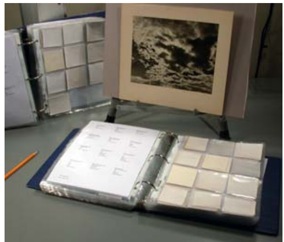
Samples of dated photographic paper in the author's collection used to assess a print of unknown origin.
