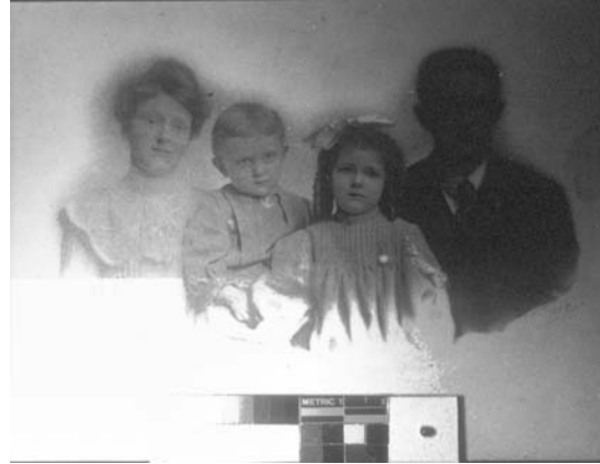
Fig. 33. Left. Reflected longwave ultraviolet photograph of a damage tintype, showing emulsion lifting and corrosion.
