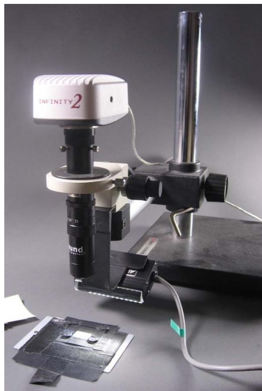
**Fig. 1. System for raking-light close-up image acquisition**
