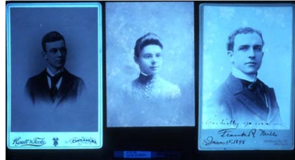
Fig. 23. Same images in fig. 22, irradiated by long wave ultraviolet, and showing the difference in visible fluorescence between albumen and collodion binders.
