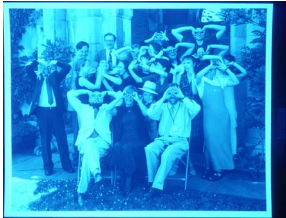
Fig. 21. Group Portrait , gelatin silver print, 9 9/16 x 7 9/16 inches, irradiated by long wave ultraviolet and showing strong visible fluorescence from optical brighteners.
