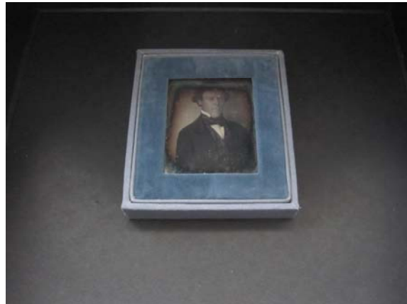
Figure 9: Plate package with corrosion inhibiting retainer in exhibition container
