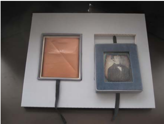
Figure 8: Plate package with corrosion inhibiting retainer in a storage container with multiple trays
